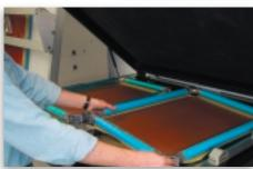
The screen is then aligned on the Tri-Loc Master Registration Frame. Three stop points assure that the screen and film are precisely and tightly locked into the desired position during vacuum pull down.
