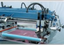
The operator simply raises the press carousel, pulls the screen into contact with the pallet's three stop points, and locks the screen into place. The result is precise and repeatable registration from print head to print head.
